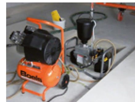
Membrane airless machine with compressor drive
