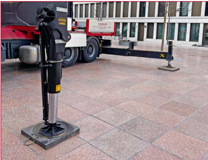
High point loads are no problem for the flexible joint
